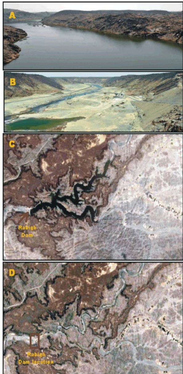
Fig. 4: Satellite images and field photos show the encouraging water potential in Rabigh basin. A: shows accumulation of large volume of water in the channel of the wadi as reservoir behind the Rabigh dam; B: shows the discharged water the spillway from the dam; C: shows extent of accumulated water in the channels of wadis, which used to serve as reservoir of the dam with reference to image of May 2014; D: shows the presence of groundwater springs within the channels of wadis flowing through basaltic lava before the completion of the dam with reference to image of July 2005. Source of images: Google earth.
