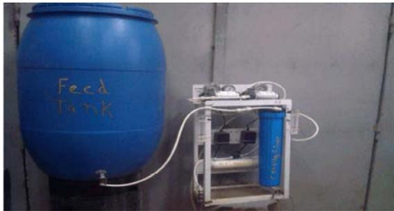
Fig. 2: Shows a photo of the entire membrane pre-treatment system
