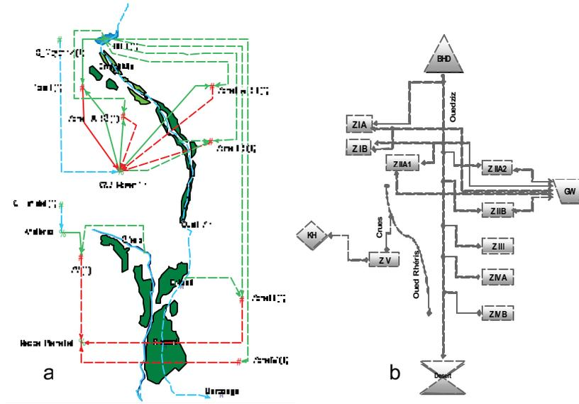
Fig. 4: a) WEAP conceptual Model for water management and irrigated area in Tafilalet, b) Water distribution in main parts of the Ziz oasis
