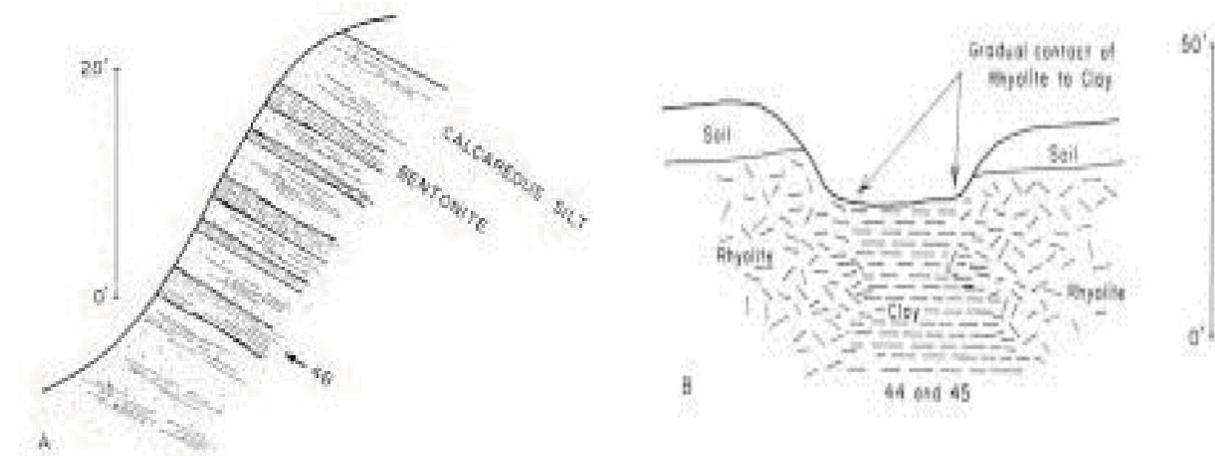
Fig. 1: Two profiles from Algerian bentonite deposits formed in different ways
