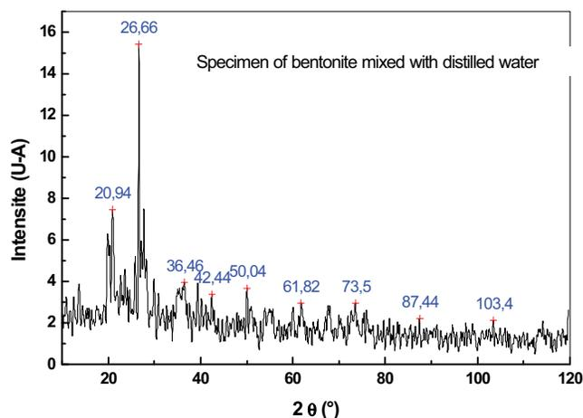
Fig. 2: X-ray diffraction spectra of the bentonite
