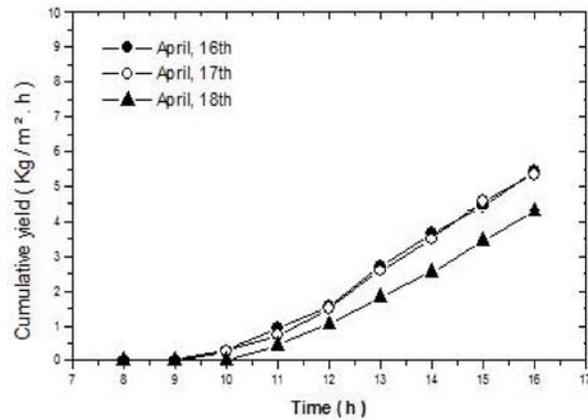
Fig. 10: Cumulate yield of Distillate versus time
