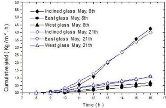
Fig. 14: Cumulate yield of Distillate versus time
