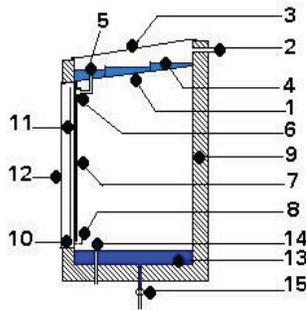
Fig. 1: schematic diagram of solar still
