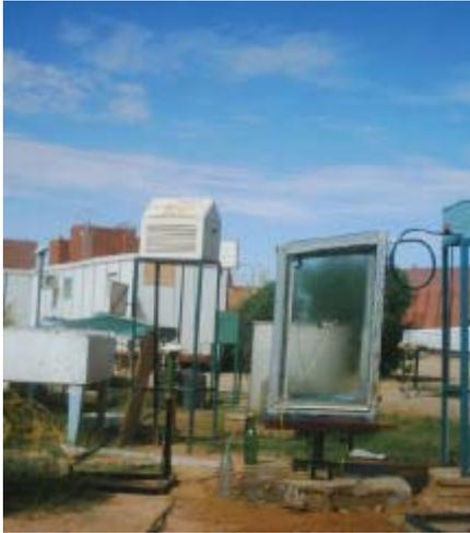
Fig. 5: Experimental set up of novel solar still
