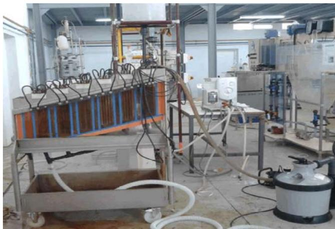
Fig. 1: Conception of unit pilot electrocoagulation
