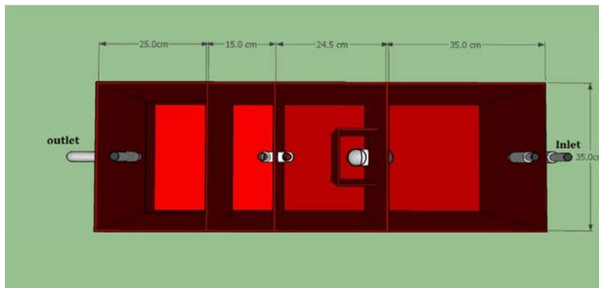
Fig. 4: Top view of the experimental unit
