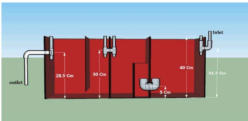
Fig. 5: Elevation of the experimental unit
